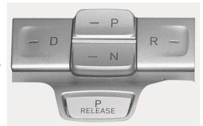
Position the shift lever in park (P)
