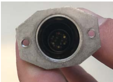
Photo 3. Failed discharge pressure transducer.
