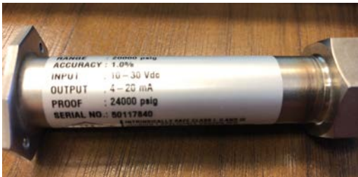
Photo 2. Failed discharge pressure transducer.
