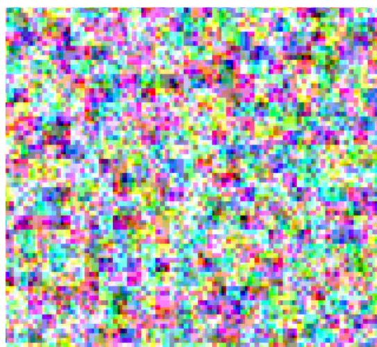
Figure 2. Dot pattern used for the BOS technique.
