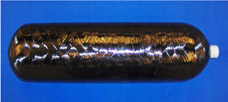
Figure 4- Composite Type 3 cylinder designed to ISO 11119-2 for WP = 232 bar
