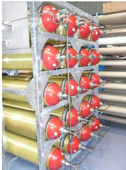
Figure 1-Composite Type 2 cylinders for stationary applications
