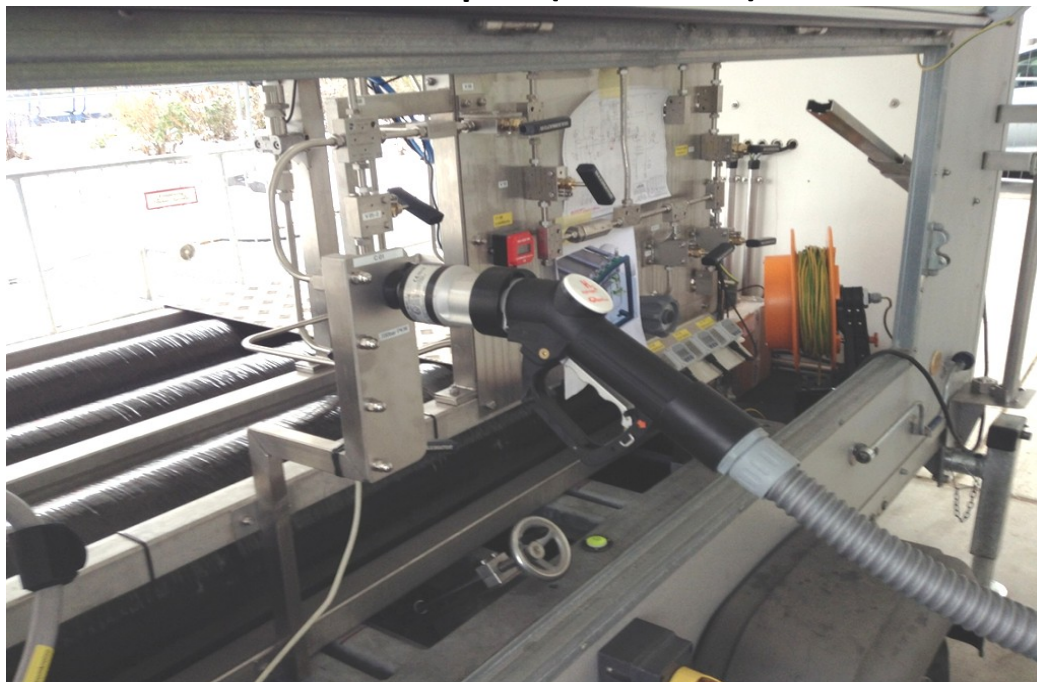
Figure 6: Example of a hydrogen station test apparatus (HSTA)
