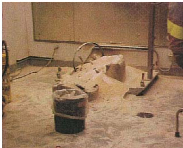
Figure 4 Sodium hydride fire extinguished with Met-L-X TM (from Fluegeman et al., 2005)
