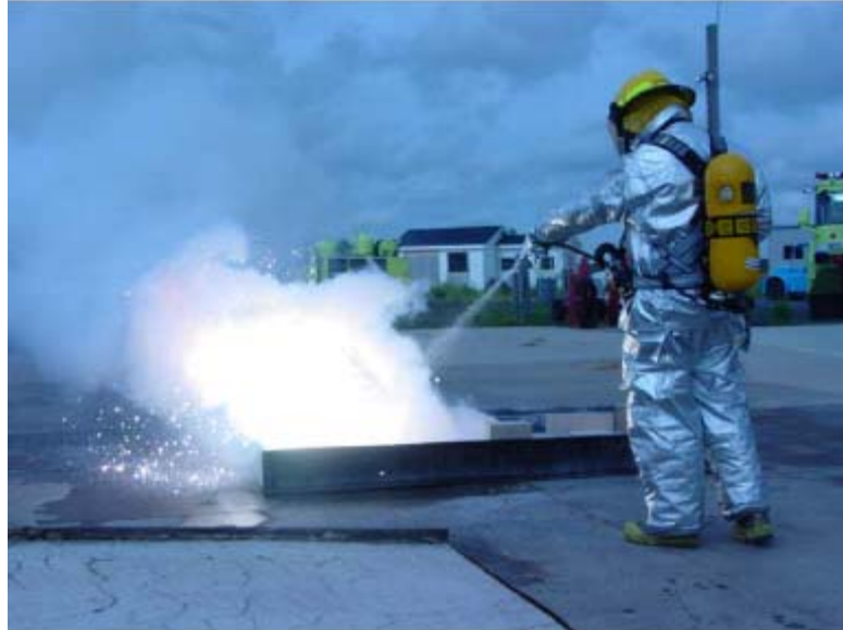
Figure 3. Application of liquid agent FEM-12 to burning magnesium (from ref 8).
