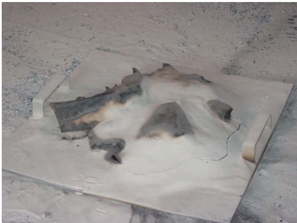
Figure 2 Results of sodium chloride based agent application to burning magnesium (from reference 8)
