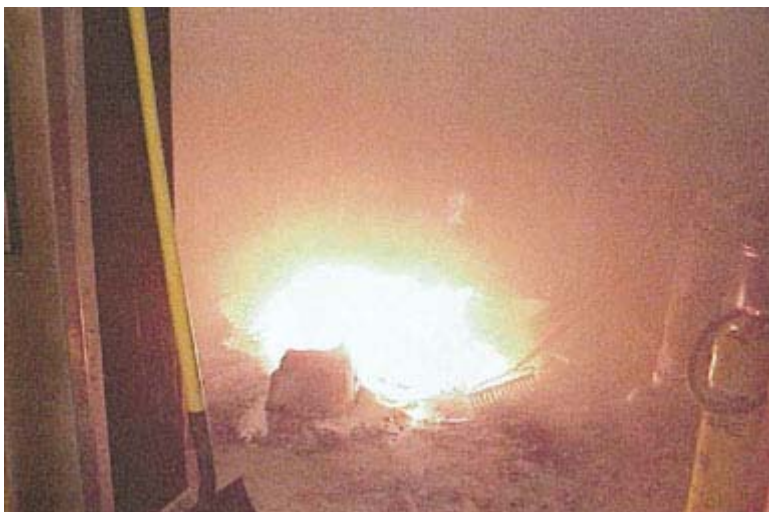
Figure 1 Controlled Sodium Hydride Fire (from Fluegeman et al, 2005)
