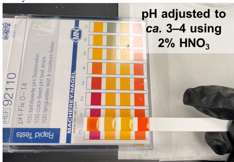
Figure 2. pH adjustment using 2% \text{HNO}_3 .
