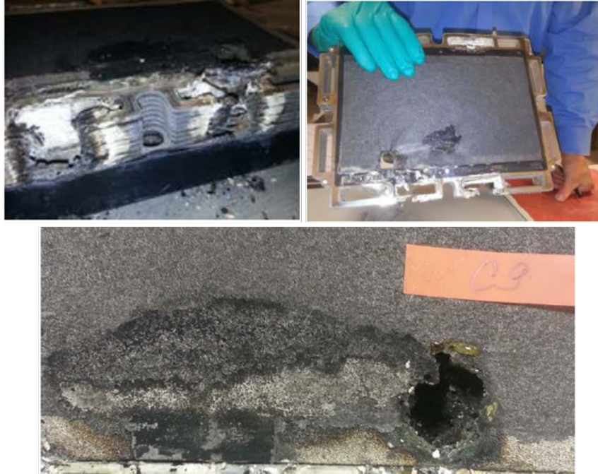
Figure 27. Crossflow condition test—internal damage to fuel cell stack
