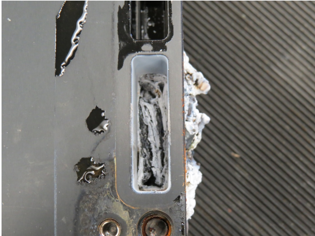
Figure 14. Loss of coolant test—post-test photograph of cathode inlet port with gas manifold removed
