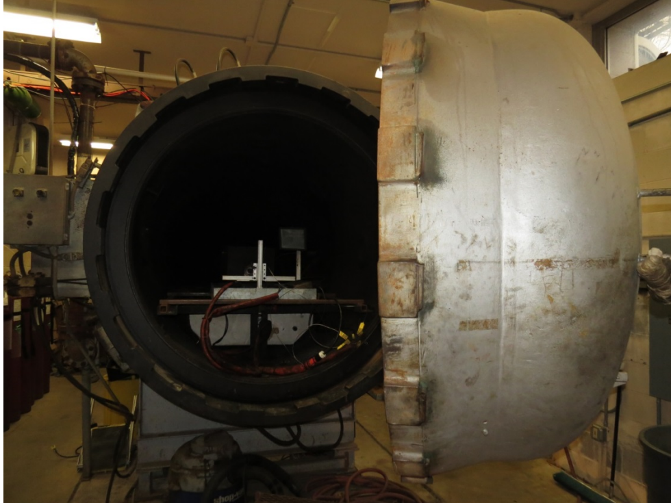
Figure 2. Pressure vessel located at the FAA's Pressure Fire Modeling Facility
