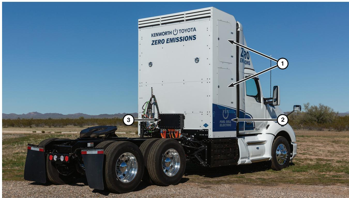
① Cabinet doors for Compressed Hydrogen Storage System (CHSS)
