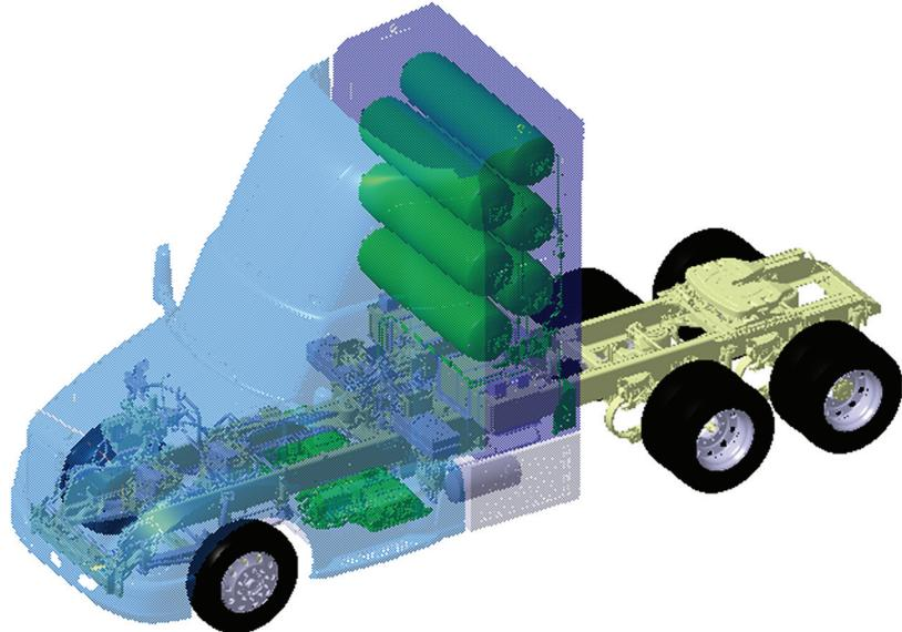
The hydrogen pipes are located in the rear cabinet and underneath the floor.
