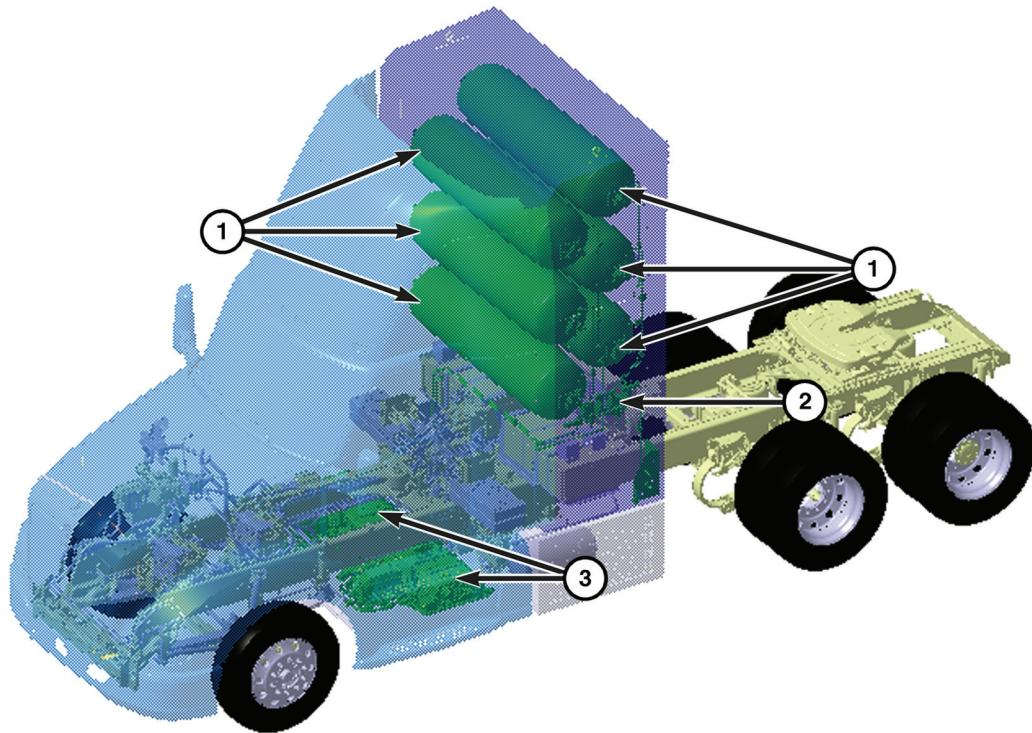
① Compressed Hydrogen Storage System (CHSS) cylinders
