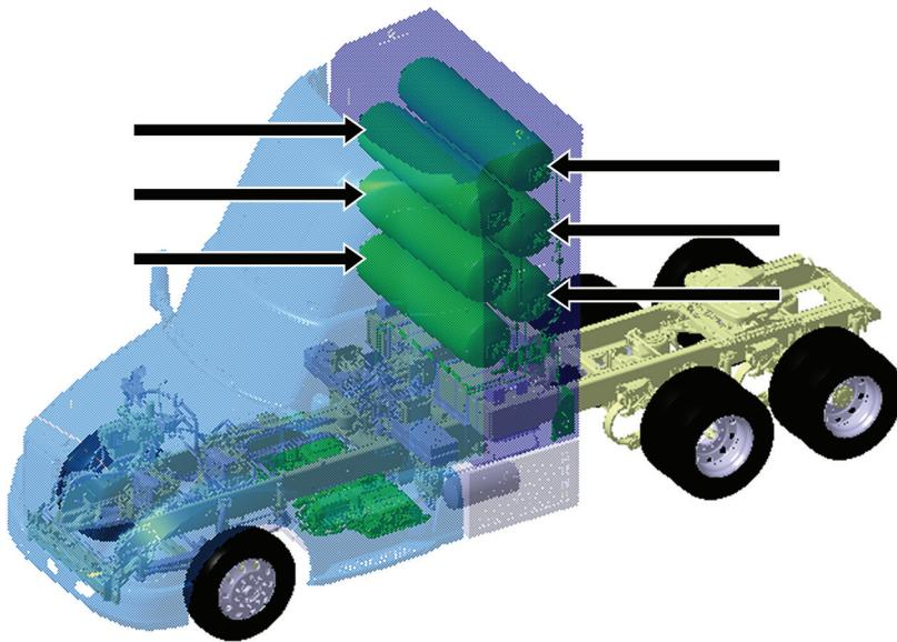
The Compressed Hydrogen Storage System cylinders are filled with high pressure hydrogen gas (nominal 10,153 psi (714 kgf/cm<sup>2</sup>, 70 MPa) at 15°C (59°F)) to supply the fuel cell stacks.
