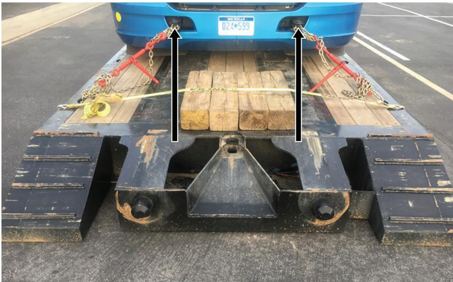
Secure the rear of the fuel cell electric truck with DOT approved series 7 chains, tied down at 45 degree angles to the rear axles, as pictured below.
