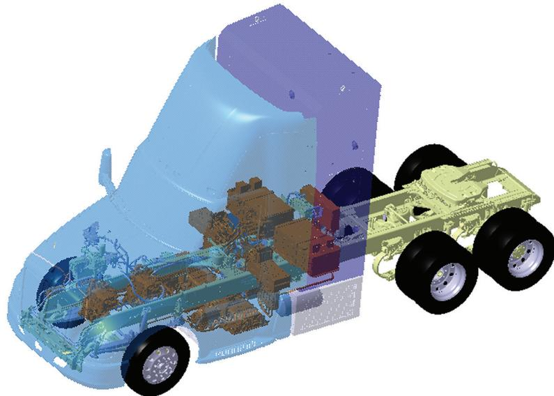
High voltage flows through heavy-duty power cables, connecting the high voltage components. High voltage cables are indicated by an orange color and are installed in the underhood compartment and toward the center of the truck (routed through the inner chassis below the cab) or on either side away from the cab and lower panels.
