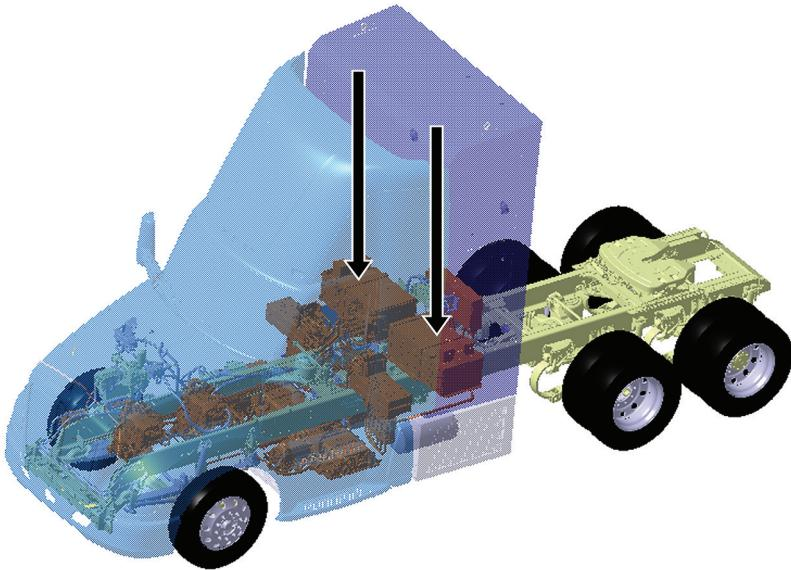
The battery electrolyte is sealed inside the high voltage battery, and a crash causing large amounts of electrolyte to spill is highly unlikely. There are 2 service plugs (300 V) located on top of each battery.
