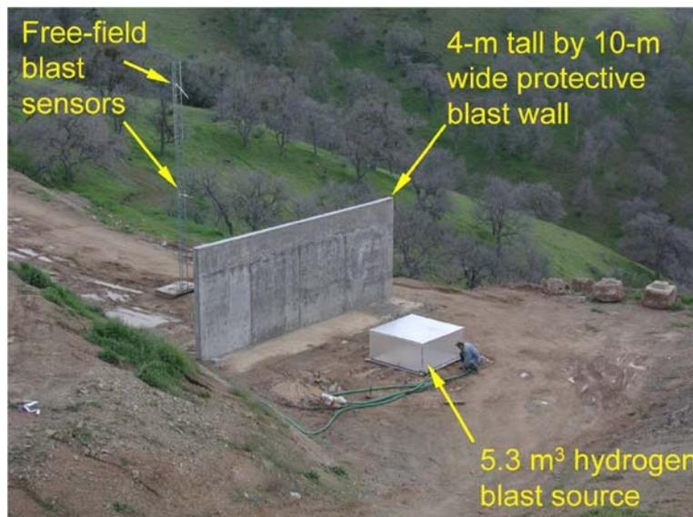
Figure 14. Protective blast wall experiment.
