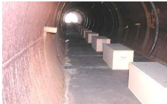
Figure 9. Model vehicles in the tunnel.
