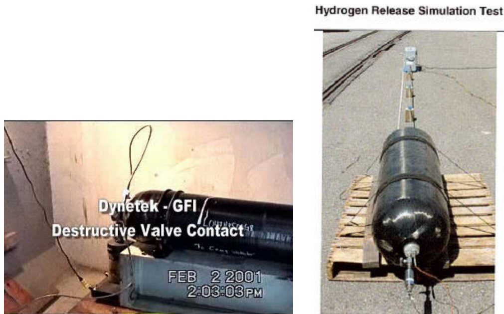
Figure 5. Examples of destructive and non-destructive experiments at Powertech Labs
