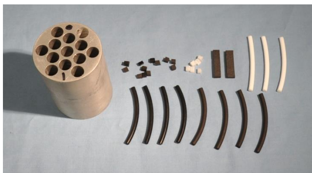
Figure 1: Sample holder and O ring specimens of polymers used in tests
