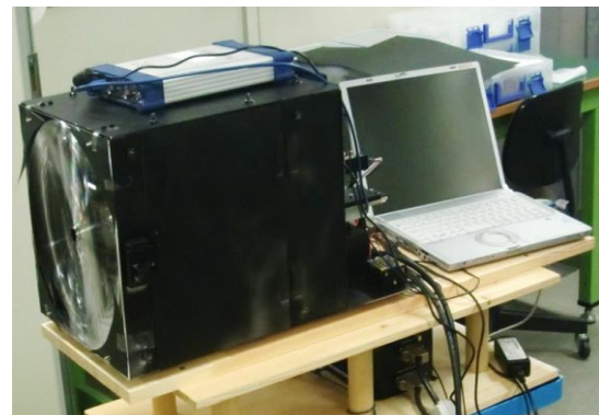
Figure 11. New Raman sensor to measure hydrogen from a distance away
