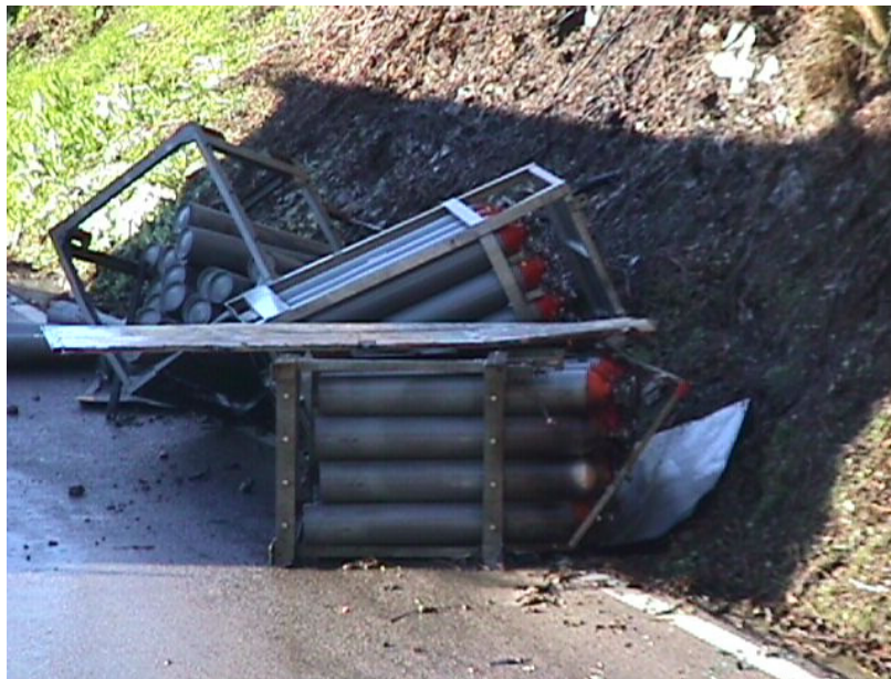
Figure 5° Packages cylinders fallen on the center road. Metallic structures of containment has collapsed.
