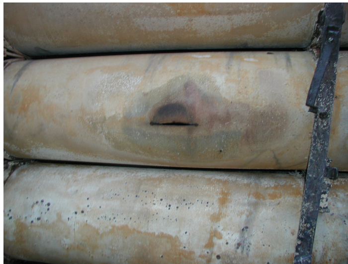
Figure 2° Hydrogen Cylinder breakup for combined effect of pressure inside and temperature.
