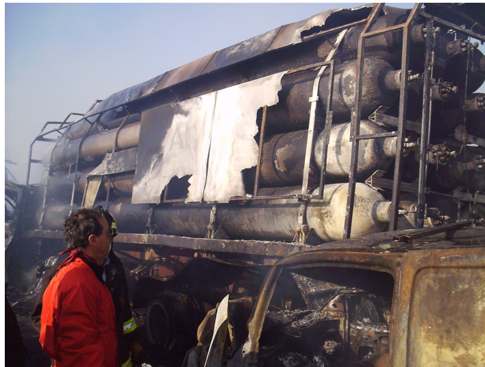
Figure 1° Hydrogen tube trailer after the accident.
