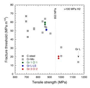
Figure 1. Fracture threshold determined from elastic-plastic fracture toughness measurements in gaseous hydrogen at pressure of 106 MPa. Carbon steel [5,6] and Cr-Mo steel [7] data from previous studies in hydrogen at pressure of 103 MPa and displacement rate of 1.5 and 3 mm/h respectively. Each data point represents an individual test.
