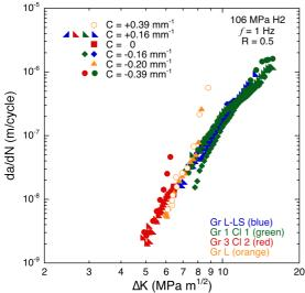
Figure 3. Fatigue crack growth rate of Ni-Cr-Mo pressure vessel steels in gaseous hydrogen at pressure of 106 MPa, with load ratio of 0.5 and frequency of 1 Hz.
