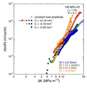
Figure 2. Fatigue crack growth rate of Ni-Cr-Mo pressure vessel steels in gaseous hydrogen at pressure of 106 MPa, with load ratio of 0.1 and frequency of 1 Hz.
