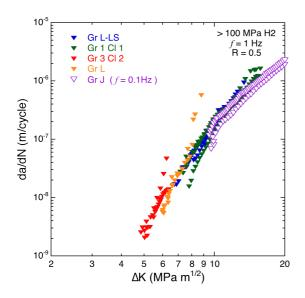
Figure 5. Comparison of fatigue crack growth rates for Ni-Cr-Mo pressure vessel steels and Ni-Cr pressure steels in high-pressure gaseous hydrogen at R = 0.5. The Ni-Cr-Mo data is from Figure 3, while the data for Cr-Mo steel represents two heats of SA-372 Grade J steel and was generated at a frequency of 0.1 Hz in hydrogen at pressure of 103 MPa from Refs. [3,4].
