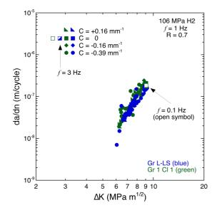
Figure 4. Fatigue crack growth rate of Ni-Cr-Mo pressure vessel steels in gaseous hydrogen at pressure of 106 MPa, for load ratio of 0.7 and frequency of 1 Hz. A few test segments were conducted at 0.1 Hz and 3 Hz, but showed no significant differences compared to test segments at 1 Hz.
