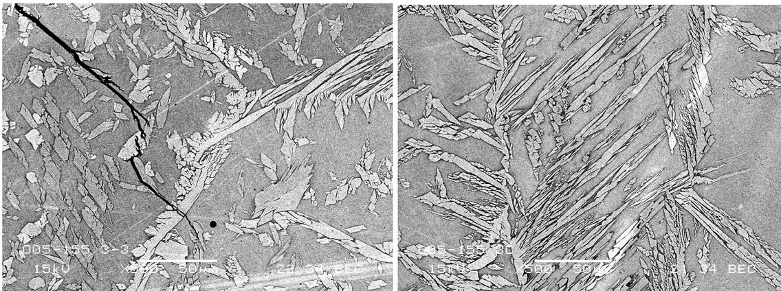
Figure 4. SEM images of duplex weld from the first tests (left, with crack) and from the repeated tests that did not show SCC (right). Light areas are austenite grains and darker areas are ferrite grains.
