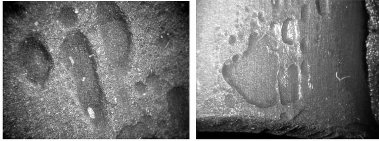
Figure 3. Local corrosion attacks on duplex 2304 exposed at 120°.
