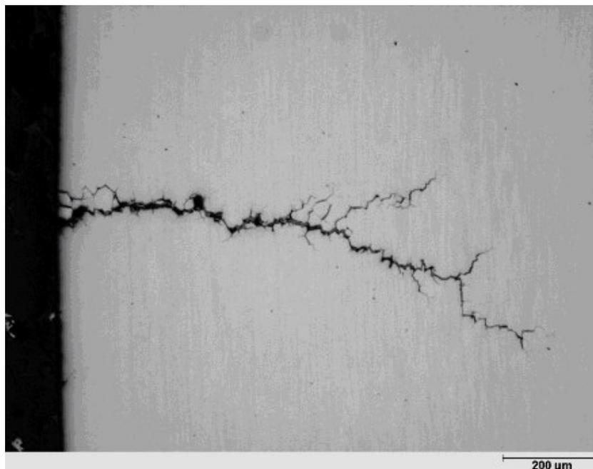
Figure 2. Cross section image of a stress corrosion crack in AISI 316L.
