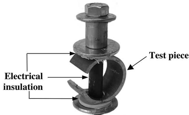
Figure 1. C-ring test specimen mounted with compression bolt and electrical insulation.
