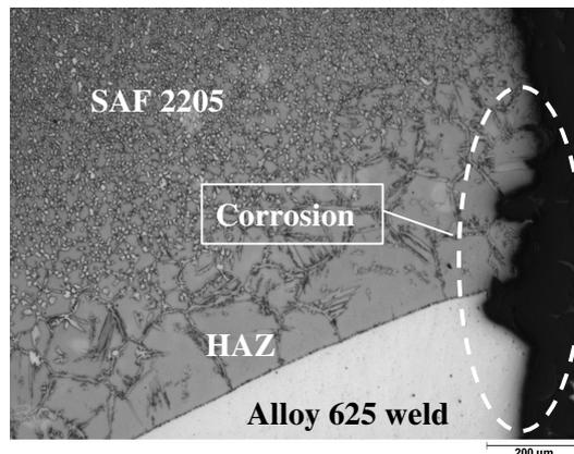
Figure 5. Duplex 2205 welded with Alloy 625 filler material showing local corrosion attacks in the transition zone between base material and weld.
