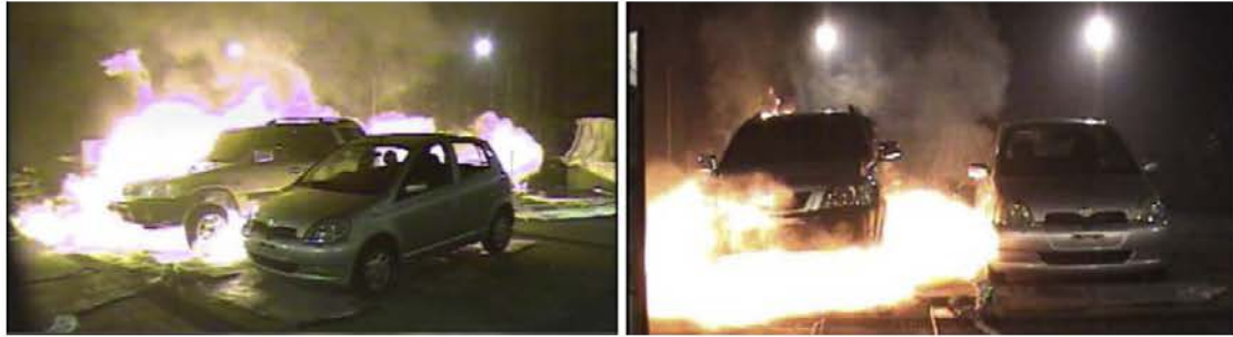
Figure 3. A snapshot of 70MPa ignited hydrogen release from a TPRD [4].
