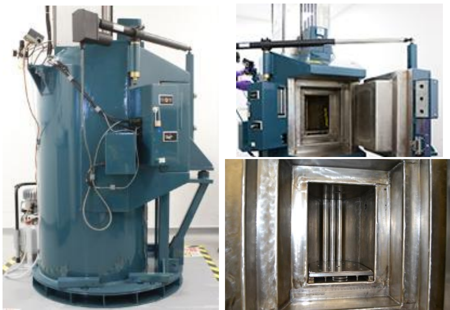
Figure 1. ^{60}\text{Co} gamma irradiator
