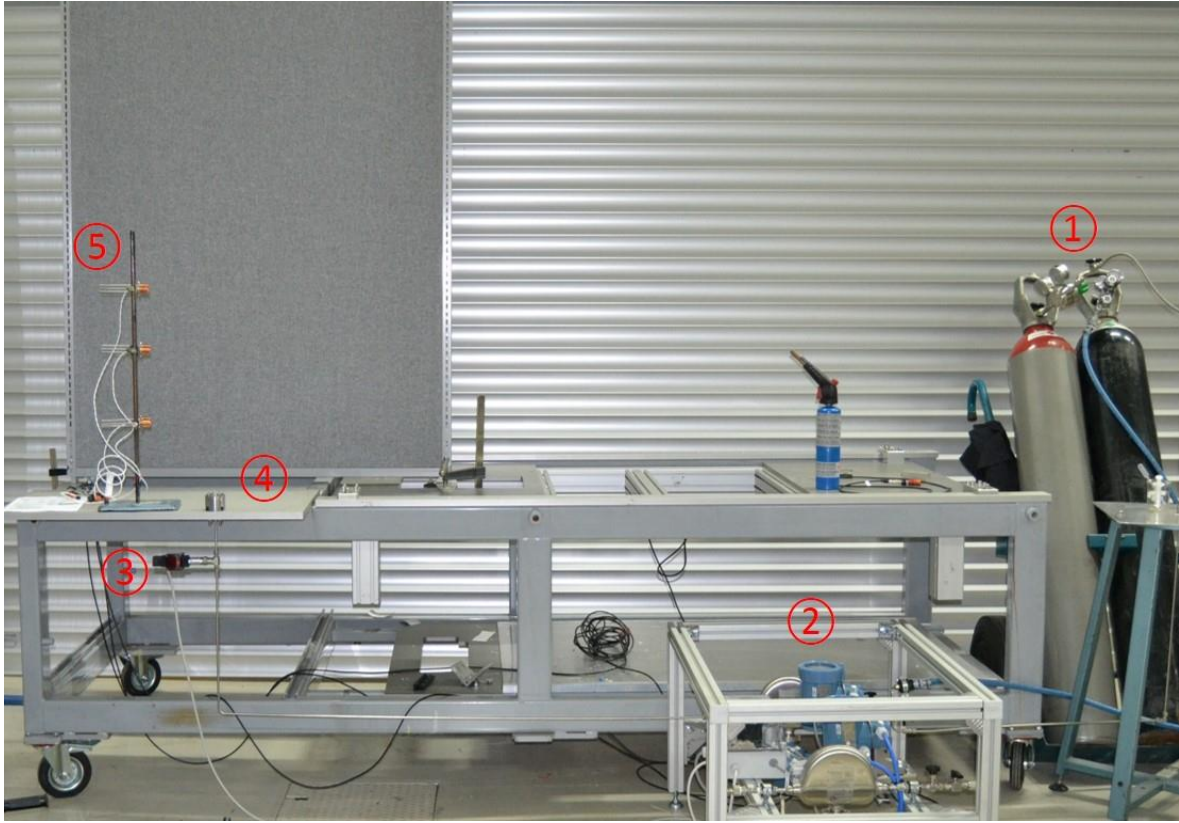
Figure 1. The experimental setup: 1) Hydrogen gas cylinder, 2) mass flow meter, 3) pressure sensor, 4) nozzle unit with changeable nozzle configurations, 5) radiation sensors (currently not in use).
