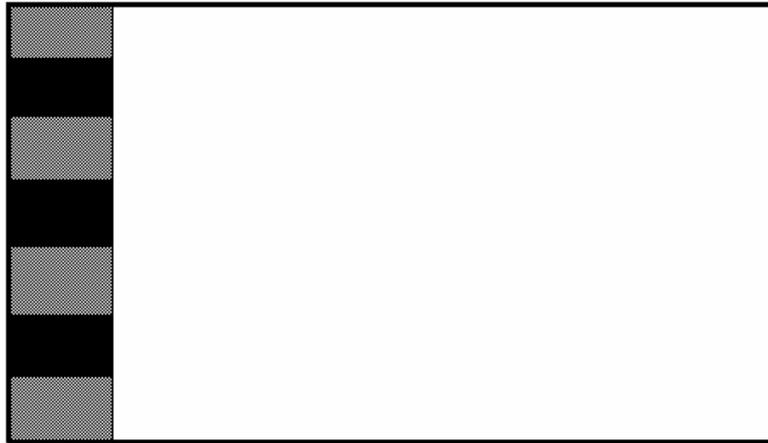
Figure 2. Initial pressure and temperature perturbation used to trigger 2D detonations waves propagation from left to right. (black zone – (1000p<sub>0</sub>(atm), 25T<sub>0</sub>(K)), grey zone – (p<sub>0</sub>(atm), T<sub>0</sub>(K))
