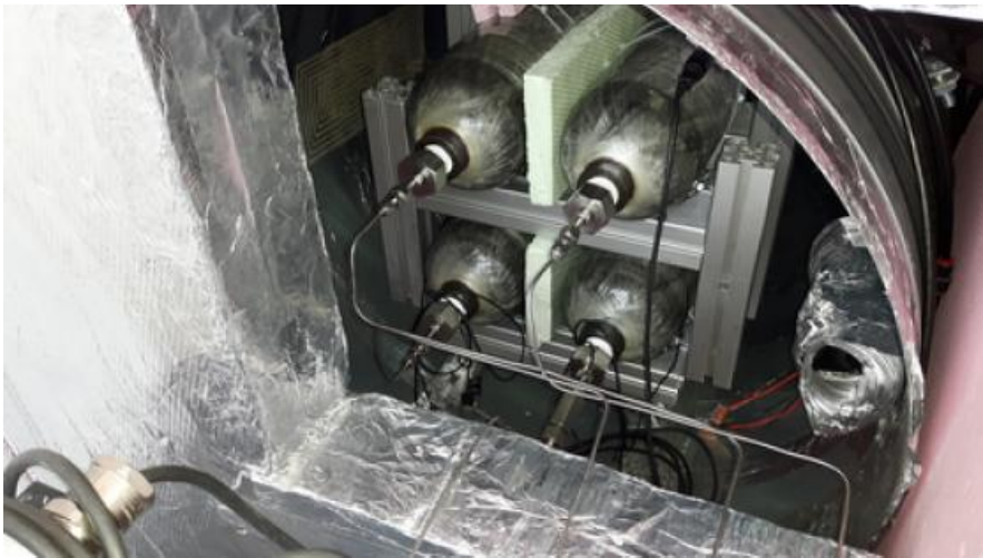
Figure 2 Picture of the experimental setup with four vessels inside the climatic chamber. A microphone and a thermocouple are placed on the external surface of each vessel.
