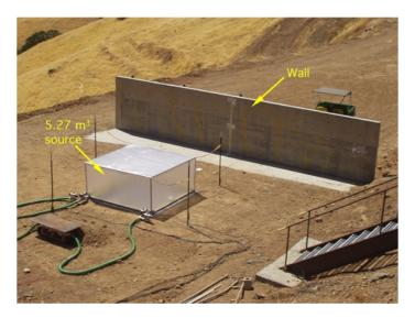
Figure 1. Wall and explosive source
