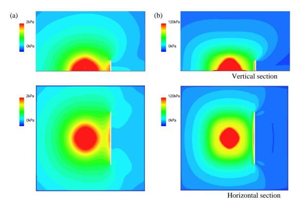
Figure 15. Distribution of the peak blast pressure around the barrier wall for (a) Case1 (b) Case2
