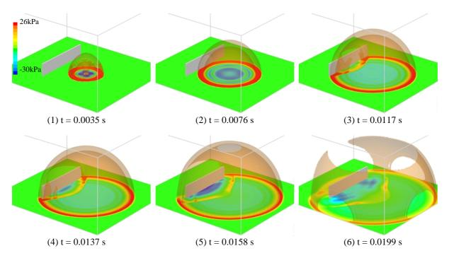
Figure 11. Instantaneous pressure contours and pressure iso-surfaces at various time steps in the detonation case (Case2)
