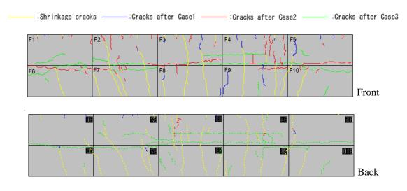
Figure 9. Distribution of cracks after each test
