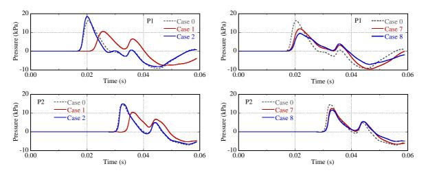
Figure 21. Blast pressure time histories at points P1 and P2
