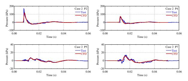
Figure 13. Blast pressure time histories on the barrier wall in Case2
