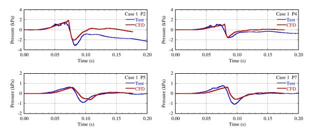
Figure 12. Blast pressure time histories on the barrier wall in Case1
