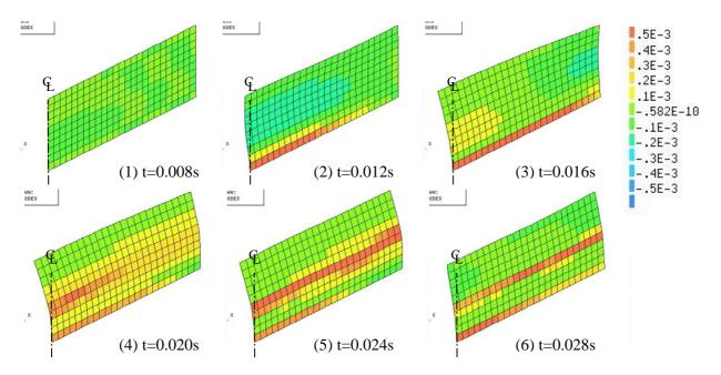
Figure 18. Concrete strains on the front surface of the wall in Case2 at various time steps
