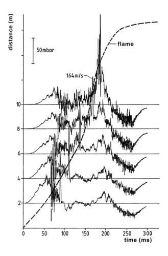
Figure 1. Flame propagation and pressure time histories for a quiescent hydrogen air mixture (37%  $H_2$ ) in a lane
