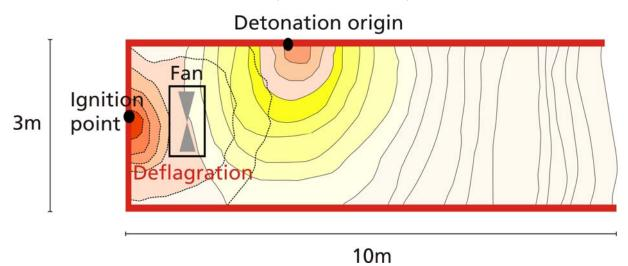
Figure 3. Propagation of flame front and detonation front in DDT experiment in a lane (turbulent hydrogen air mixture with 37% H<sub>2</sub>)
