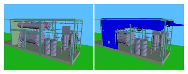
Figure 4. Visualisation of the gas dispersion model of the hydrogen production container (without cladding). Left: Before leakage. Right: Extents of lower flammability limit for hydrogen/air mixture inside container after 60 seconds.
