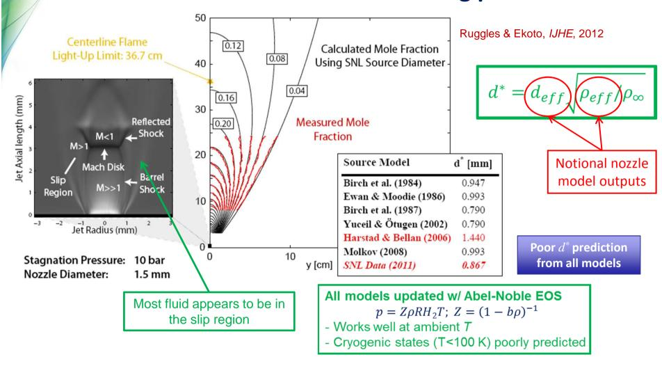
Unclear if equivalent diameters can be used for slot nozzles
