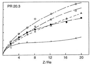
Elevated near field jet area ratios result in faster initial concentration decay rates
