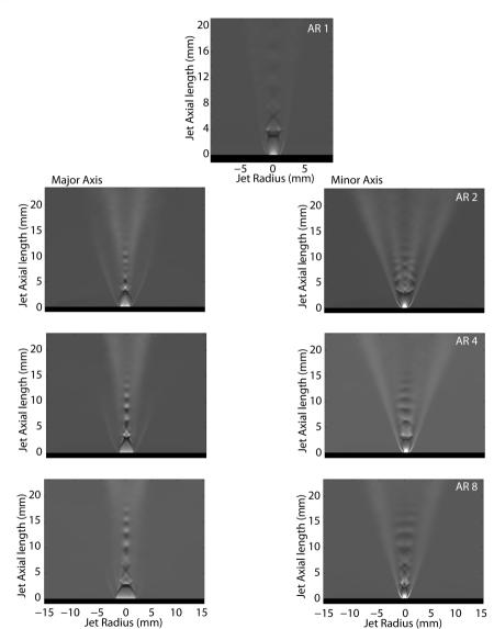
Downstream oblique shock structure disappears ~12-17 mm downstream
