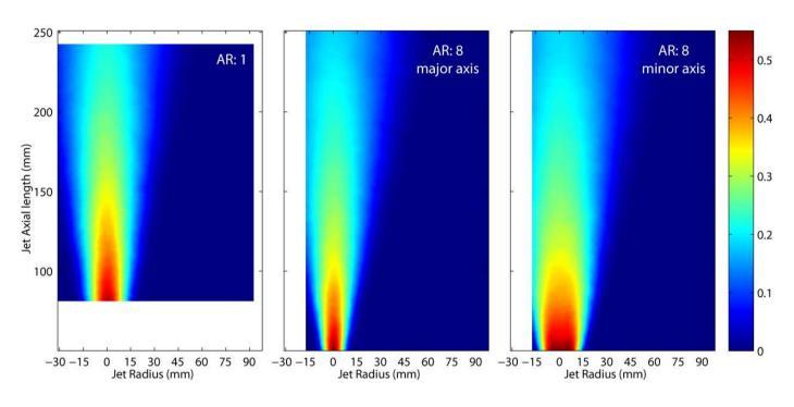
Elevated downstream mass fraction contours for the axisymmetric jet
