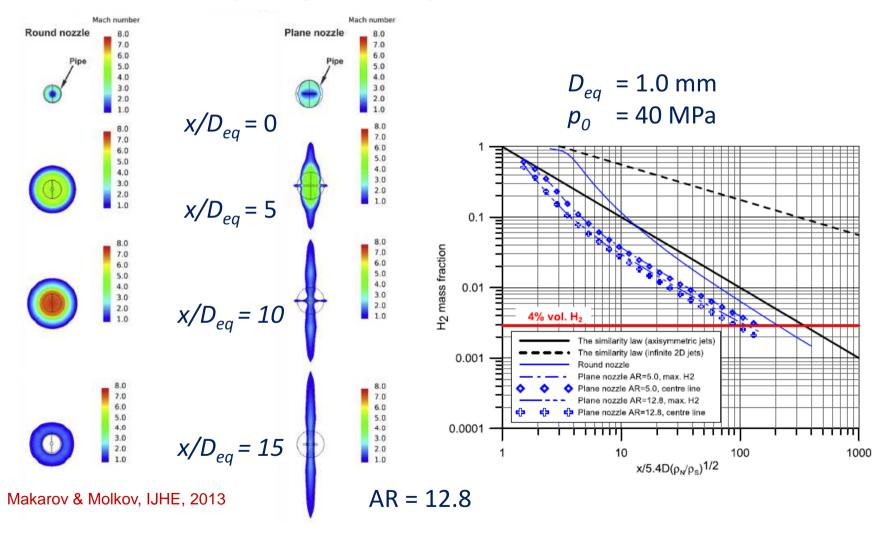
Faster slot jet centerline decay rates due to increased area available for entrainment
