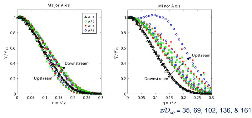
Minor axis peak H<sub>2</sub> *near-field* concentrations observed away from the centerline – not predicted by planar integral models
