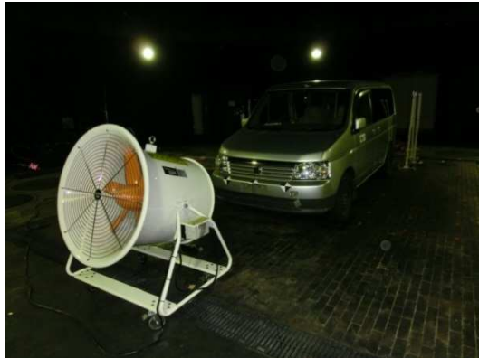
Blower 2 m forward to vehicle; wind velocity distribution on vehicle front
