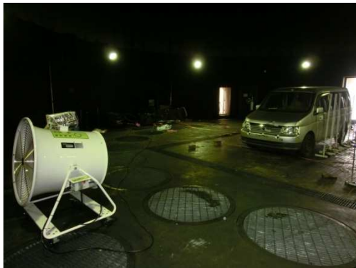
Blower 5 m forward to vehicle; wind velocity distribution on vehicle front
