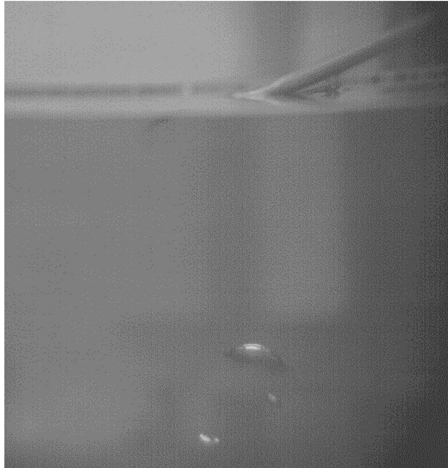
2 \text{ cm}^3 \text{ H}_2 bubble rising to a water surface length of video clip 600 ms
