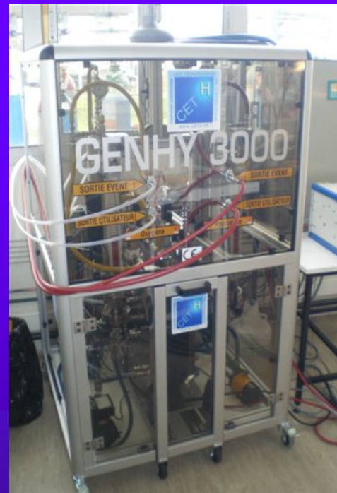
GenHy ® 3000 NI H 2 /hour max input = 5 kW 1-50 bars
