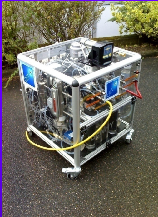
GenHy ® 1000 NI H 2 /hour max input = 5 kW 1-10 bars
