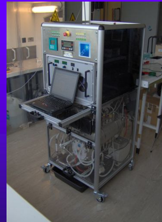
GenHy ® 5000 NI H 2 /hour max input = 30 kW 1-10 bars
