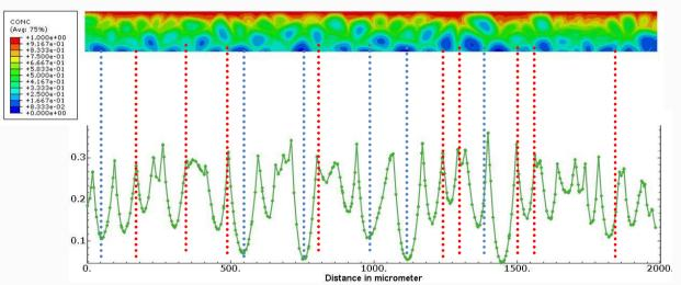
Inhomogeneous behaviour of hydrogen transport and accumulation in polycrystalline material between intergranular region and grain region with smaller grain size.
