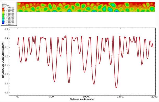
Inhomogeneous behaviour of hydrogen diffusion and accumulation in polycrystalline material between intergranular region and grain region with bigger grain size.
