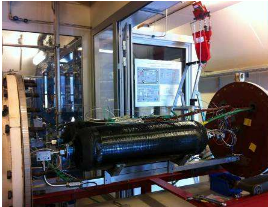
Tank internal and external instrumentation before start of the cycling
