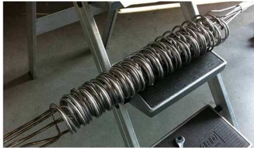
Hydrogen pre-cooler based on liquid nitrogen immersion
