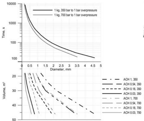
Figure 5. Nomogram for 1kg, 350 and 700 bar.
