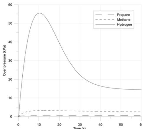
Figure 1. Pressure dynamics in a 30.4 m<sup>3</sup> garage, with a single vent, for a constant mass flow release of hydrogen, propane and methane, from 350 bar storage through a 5.08 mm diameter.
