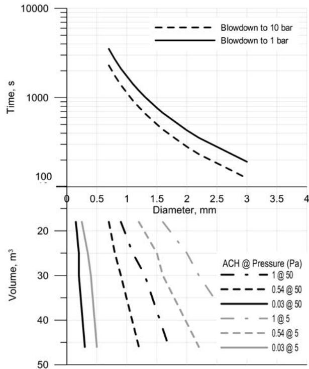
Figure 8. Nomogram for 5 kg of hydrogen at 350 bar, blowdown time to 1 bar overpressure in the storage tank, ACH calculated using  $\Delta P = 50$  Pa and  $\Delta P = 5$  Pa.
