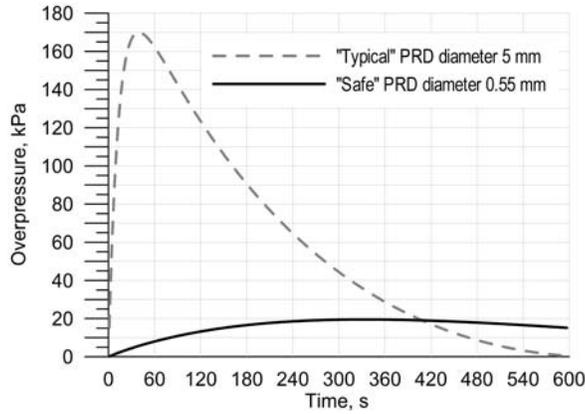
Figure 2. Pressure dynamics in a 30 m<sup>3</sup> garage, ACH = 0.18, 5 kg of hydrogen at 350 bar, diameters of 5 mm and 0.55 mm.
