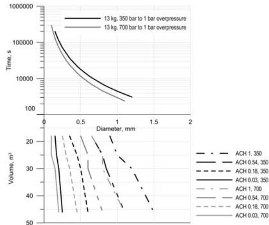
Figure 7. Nomogram for 13 kg, 350 and 700 bar.
