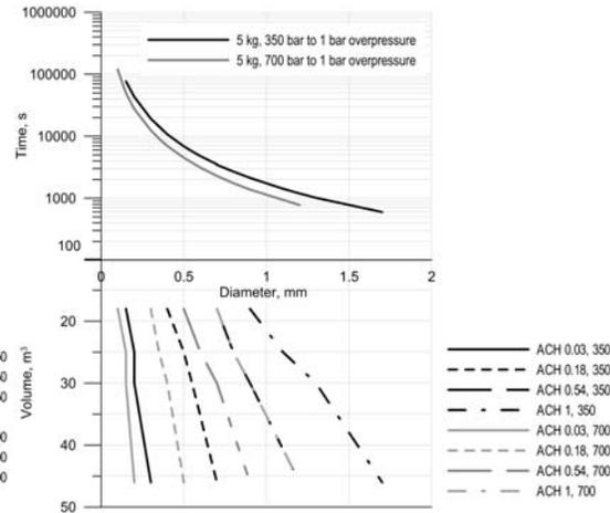
Figure 6. Nomogram for 5 kg, 350 and 700 bar.
