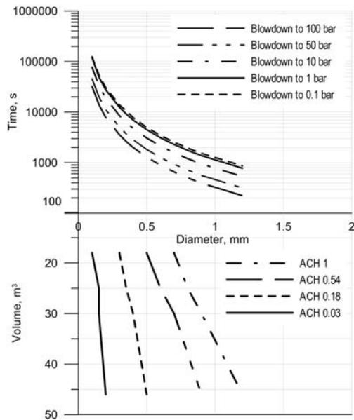
Figure 3. Nomogram for 5 kg hydrogen at 350 bar. Figure 4. Nomogram for 5 kg hydrogen at 700 bar.
