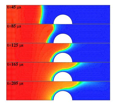
Figure 6: Temperature contours evolutions due to flame propagation. Red color corresponds to burnt gases (2387K < T < 2520K), blue color - to fresh gases (300K < T < 312K). Fine mesh.
