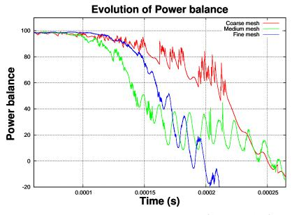
Figure 7: Variation of the power balance with time,  $\frac{(Q_{generated} - Q_{lost})}{Q_{generated}} \times 100\%$ .
