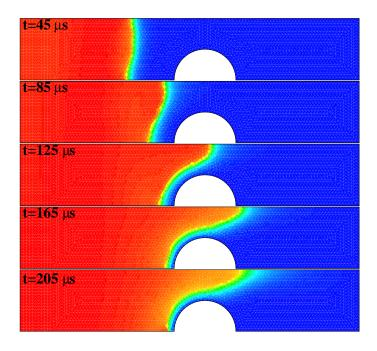
Figure 5: Temperature contours evolutions due to flame propagation. Red color corresponds to burnt gases (2387K < T < 2520K), blue color - to fresh gases (300K < T < 312K). Medium mesh.
