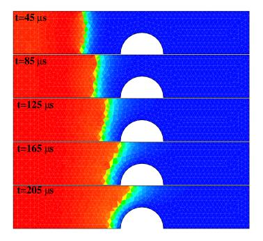
Figure 4: Temperature contours evolutions due to flame propagation. Red color corresponds to burnt gases (2387K < T < 2520K), blue color - to fresh gases (300K < T < 312K). Coarse mesh.
