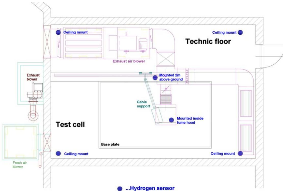
Figure 6: Sample layout of ventilation and gas monitoring system for engine test cell [3]
