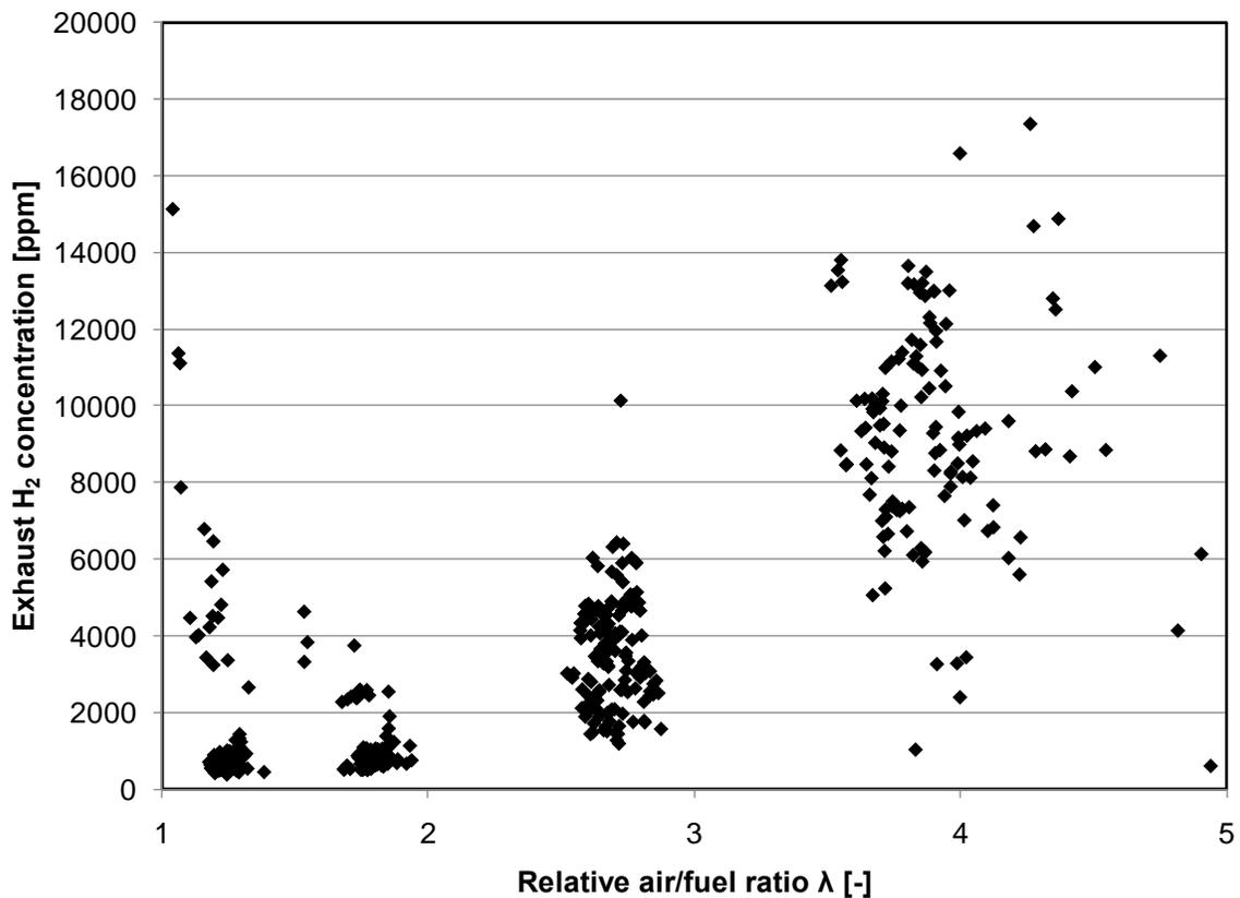
Figure 4: Exhaust hydrogen concentration versus relative air/fuel ratio
