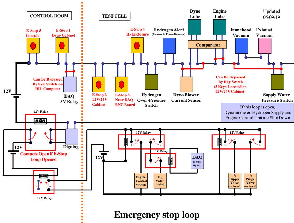
Figure 5: Sample emergency stop loop for hydrogen test cell
