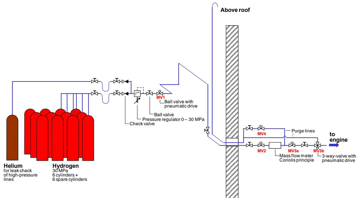
Figure 2: Sample hydrogen supply system [3]
