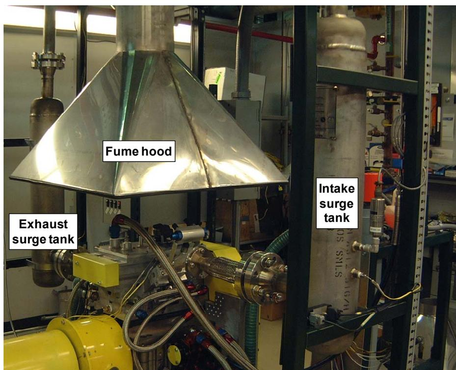
Figure 10: Pressure vessels for hydrogen intake and exhaust systems
