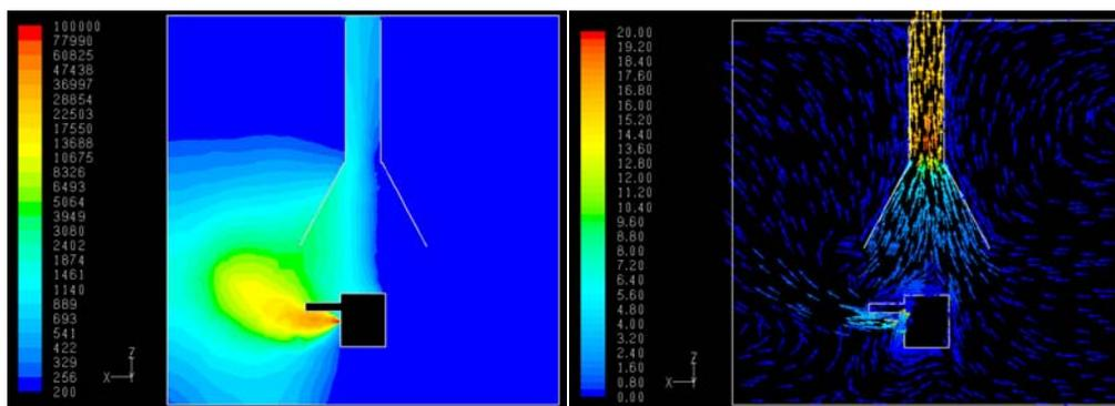
Figure 9: Hydrogen concentration in ppm and local velocities in m/s for hydrogen release scenario
