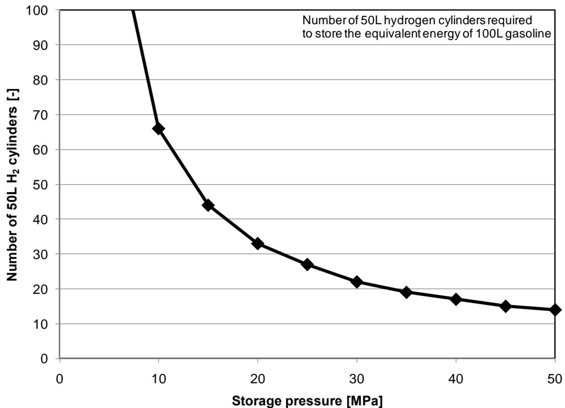
Figure 1: Estimate of compressed hydrogen storage requirements
