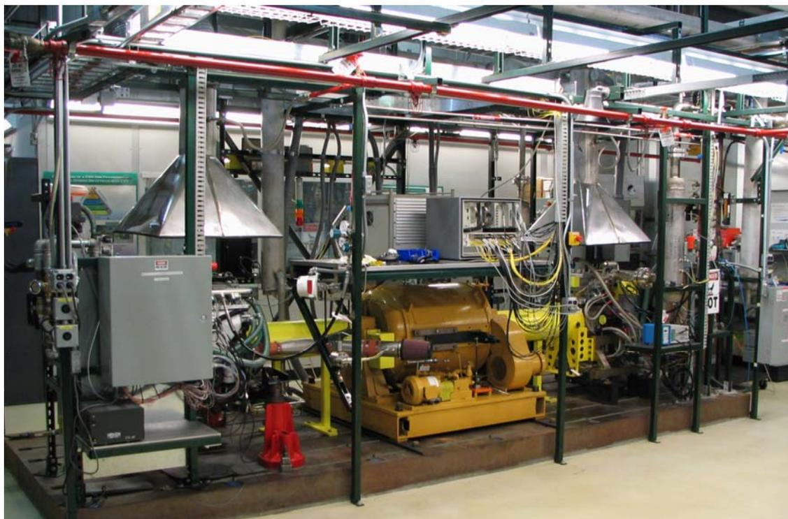
Figure 7: Dedicated hydrogen engine test cell [15]
