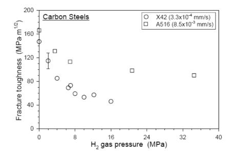
Figure 8: KIC for carbon steels. Fracture toughness decreases significantly at low hydrogen pressure before reaching a limiting value [10]
