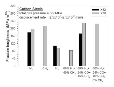
Figure 15. Fracture toughness vs. gas composition for two carbon steels [10]
