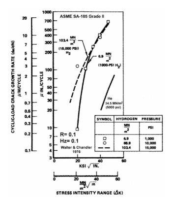
Figure 14. FCGR vs. stress intensity for SA-105 steel at 6.9 and 103.4 MPa [17]
