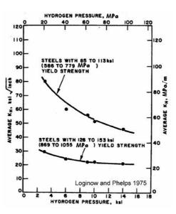
Figure 5: Influence of hydrogen pressure on threshold stress intensity factor at crack arrest [17]
