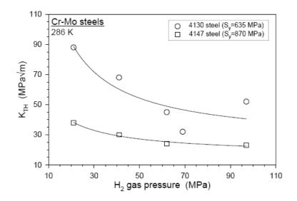
Figure 7. KTH for two ferritic steels. HE appears to have little effect on type 4147 at pressures higher than 60 MPa [10]
