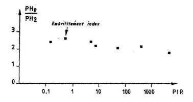
Figure 1. Effect of Pressure Increase Rate (PIR, in bar/min.) on the embrittlement index of an unspecified steel during disk rupture testing [2]
