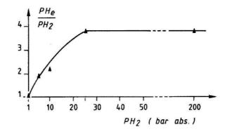
Figure 2. Effect of hydrogen partial pressure on the embrittlement index of AISI 321 steel [2]
