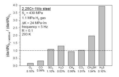
Figure 16: Ratio of FCGR with impurities to FCGR in pure hydrogen at fixed pressure and stress intensity range for a low-alloy ferritic steel [10]
