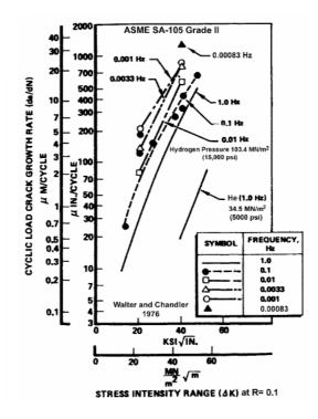
Reported effects of pressure on fatigue crack varied throughout the literature. H. Barthélémy and G.M. Pressouyre [1] provided data from tests performed by British Steel on 1% Cr-Mo steel at 1 Hz which demonstrated a clear increase of FCGR in hydrogen from 41 to 152 bar, but no significant difference between 1 bar compared to 41 bar.
