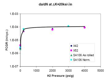
**Figure 13:** FCGR vs. Pressure for several carbon steels at  $\Delta K = 20 \text{ ksi} \sqrt{\text{in } [8]}$
