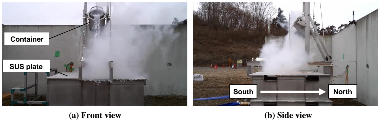
Figure 1 Image of liquefied hydrogen spilling test (with liquefied hydrogen flowing out on the SUS plate).
