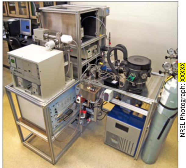
Figure 3: The NREL Sensor Test Apparatus for basic sensor performance assessment was commissioned in 2009
