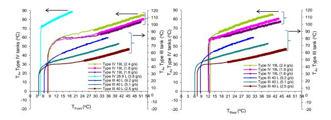
Figure 5. Correlation between tank average gas temperature  $T_{Av}$  and the temperature of (a) the front bosses  $T_{Front}$  and (b) the rear bosses  $T_{Rear}$  during the filling phase. Each curve represents one mass flow rate. Gas temperatures of Type IV tanks are given on the left y-axis while those of Type III tanks are plotted on the right y axis, for each of the two graphs. The thicker parts of each curve indicate the linear behaviour of  $T_{Front}$  and  $T_{Rear}$ .
