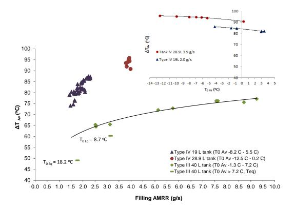
Figure 3. Effect of filling rate and tanks initial temperature on the gas average temperature increase during the filling of Type IV 19L, Type IV 28.9L and Type III 40 L tanks. The lines are guide for the eye.
