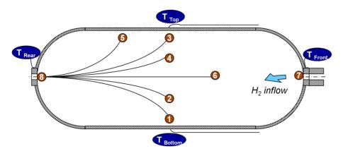
Figure 1. Arrangement of the temperature measurement instrumentation in the tested tanks
