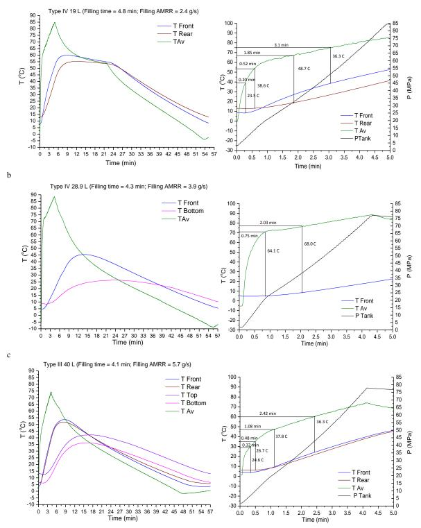
Figure 4. Evolution of the external tanks temperatures ( $T_{Front}$ ,  $T_{Rear}$ ,  $T_{Top}$  and  $T_{Bottom}$ ) and the average gas temperature during a hydrogen cycle with similar filling times (between 4 and 5 minutes) and emptying rates (between 0.3 and 0.5 g/s); (a) Type IV 19 L tank (b) Type IV 28.9L tank and (c) Type III 40 L tank.
