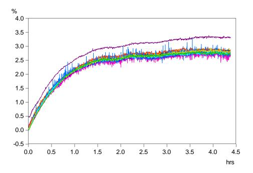
Figure 7 shows a typical set of traces recording H2 concentration as a function of time, with the hydrogen concentration settling to a steady value. One trace clearly has an offset and was omitted from the subsequent analysis.
