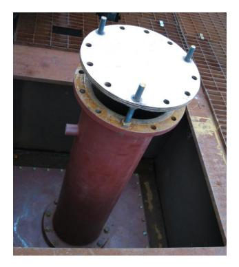
Figure 4: A 300 mm diameter chimney fitted to the top of the tank, showing the hydrogen sensor connection boss and the wooden cap.
