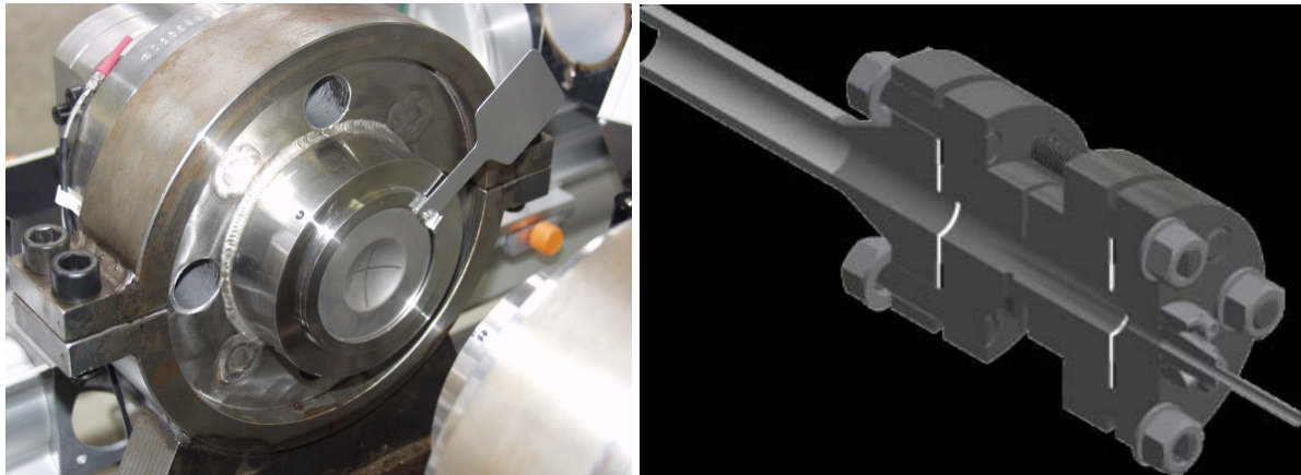
Figure 3: Rupture disc in front of the nozzle and scheme of the front end device
