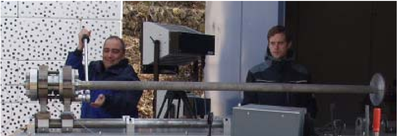
Figure 2: 5 l reservoir usable up to 400 bar to generate hydrogen jets emitted at the left end
