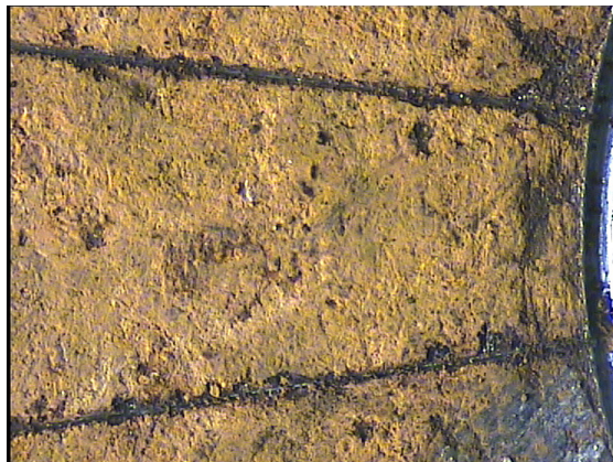
Figure 2. Naturally rusted surface produced by exposure to central London weather for several months. Magnification x 16.
