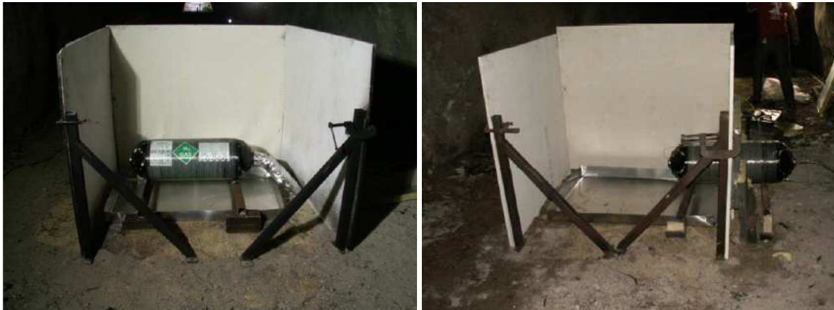
Figure 3: Experimental apparatus for bonfire tests (on the left: global fire – on the right: partial fire)
