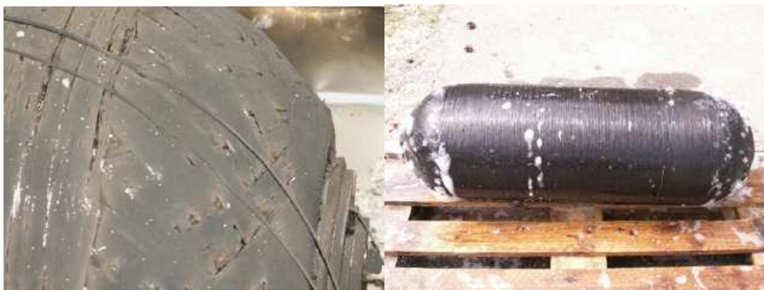
Figure 9: Cylinder P_{ini}=178 bar after bonfire test (left) and during leak test (right)
