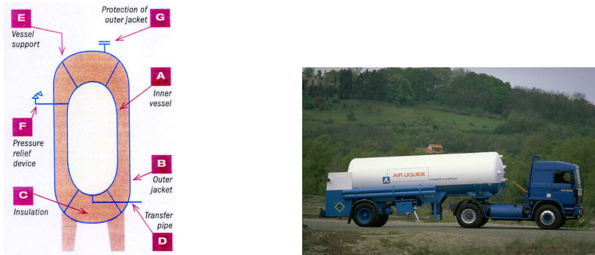
Figure 8. Cryogenic vessels: schematic and cryogenic trailer
