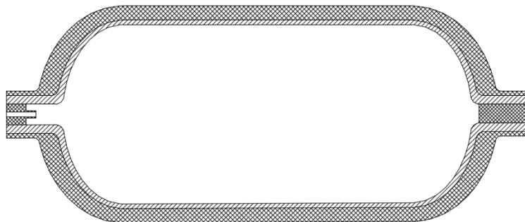
Figure 2. Structure diagram of the 70MPa vehicle cylinder
