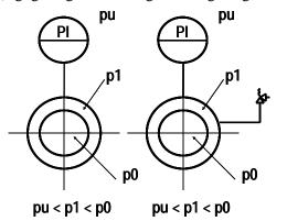
Figure 4. Sketches of Double-Walled-Pipes
