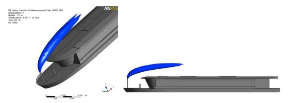
Figure 7. Example of a vent line of an inland navigational vessel
