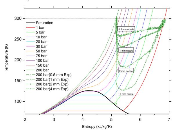
The less nozzle diameter and the longer the blow down process, the lower the temperature when non adiabatic effect or entropy deviation appears (at 200 bar):
