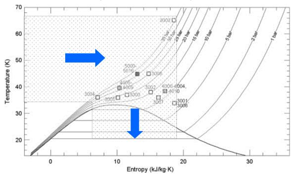
Problems to be solved: nonideality of the blow-down process (two-phase flow); non adiabatic character of the discharge process
