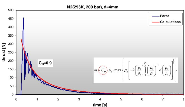
Experimental data on thrust measurements fit very well with theoretical calculations using the same discharge coefficient as for pressure dynamics
