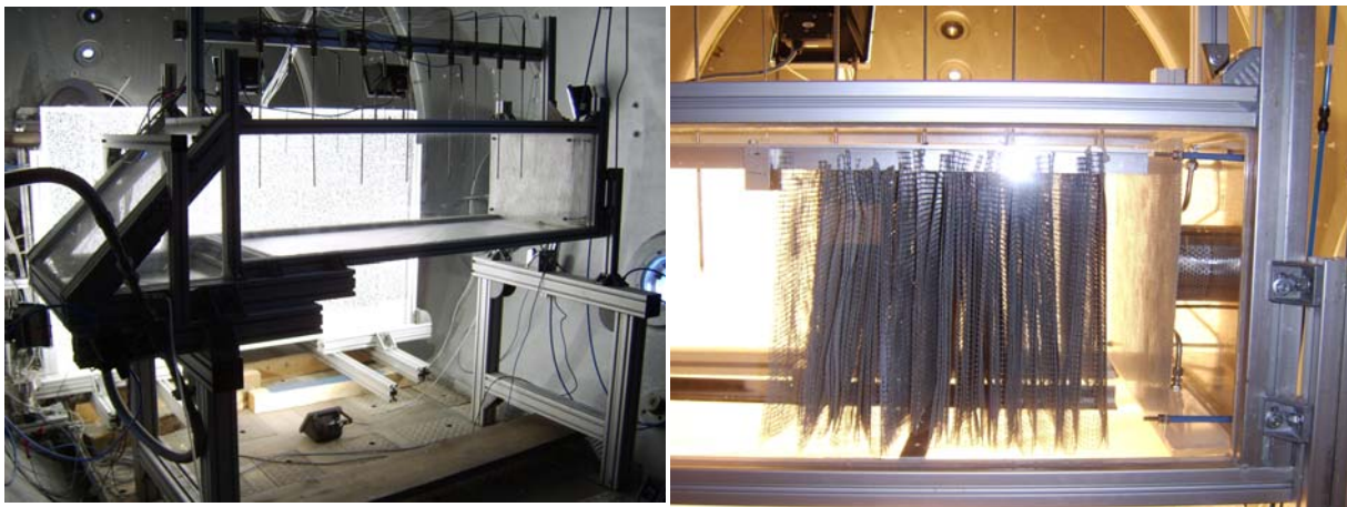
Figure 2. Photographs of the unobstructed channel (left) and the flame distributor and the grid layers installed in later experiments (right).
