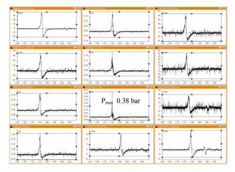
Figure 9. Pressure records of all gauges, experiment #58
