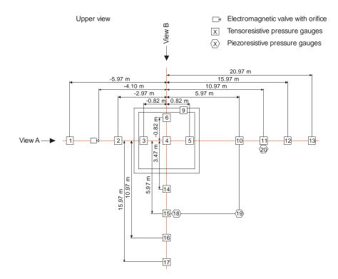
Figure 5. The scheme of locations of pressure gauges in experiments.
