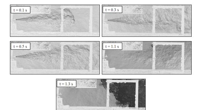
Figure 7. Sequence of BOS-photos of experiment #64 (M<sub>H2</sub>=203 g, W<sub>aver</sub>=188 g/s).
