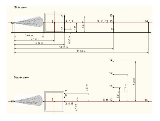
Figure 4. The scheme of hydrogen concentration sensors location in experiments.
