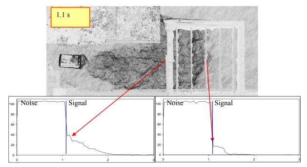
Figure 16. BOS photo after end of injection and concentration gauges records, experiment #55
