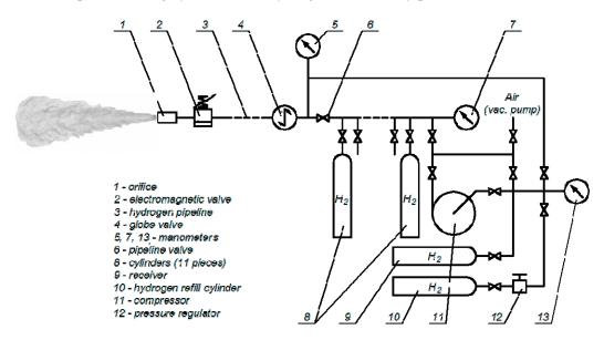
Figure 3. System of hydrogen supply.
