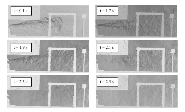
Figure 6. Sequence of BOS-photos of experiment #65 (M<sub>H2</sub>=402 g, W<sub>aver</sub>=193 g/s).
