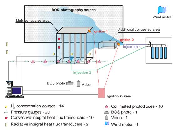
Figure 1. Scheme of experimental facility.
