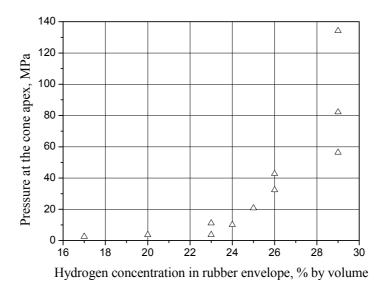
Figure 5. Maximum pressure as a function of  $H_2$  concentration in the rubber envelope. Concentration of  $H_2$  in the cone is equal 29% by volume. Initiation was made by blasting 0.8 g of PETN.
