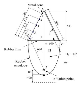
Figure 2. Scheme of Konus-2 setup. *1-6* – pressure sensors, 7 – slit inspection window for high-speed photography (all dimensions are in millimeters)
