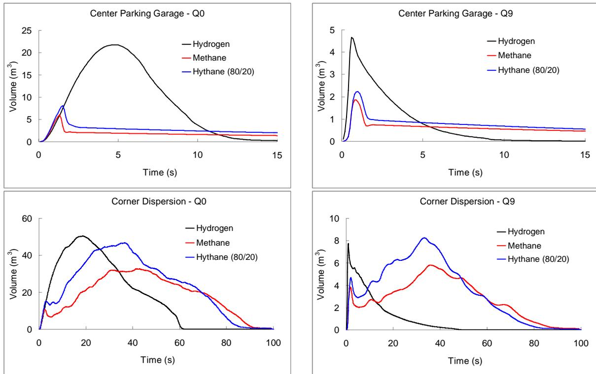
Figure 9 Total flammable volume (left) and equivalent stoichiometric gas cloud Q9 (right) for the centre (upper) and corner release scenario (lower). The total and equivalent Q9 flammable volumes for hydrogen are scaled down by a factor of 10 for both scenarios.
