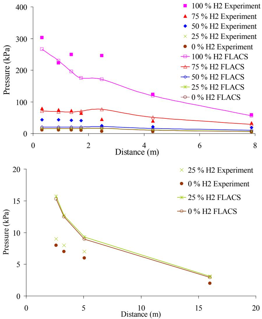
Figure 2 Pressure recordings (filled markers) versus FLACS simulations (lines) in monitor arrays parallel (M1-M7) parallel to the wall (top) and sensors away from wall (M8, M9, M10 and M15) (bottom) for methane- and hythane-air mixtures. Experimental observations are found in [6].
