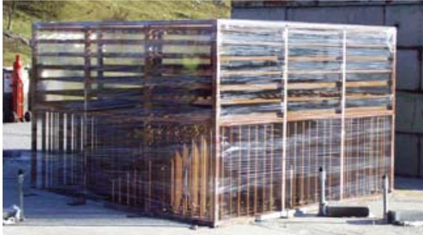
Figure 1 Overview of the pipe array, vertical wall to the right, and monitor arrays parallel (M1–M7) and perpendicular (M8–M10, M15) to the wall.
