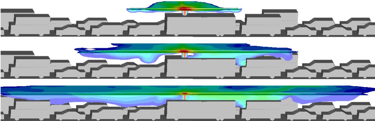
Figure 11 Hydrogen volume fractions in the tunnel geometry 1 s (top), 4 s (middle) and 12 s (bottom) after the beginning of the release. Concentrations around stoichiometry are shown in green.
