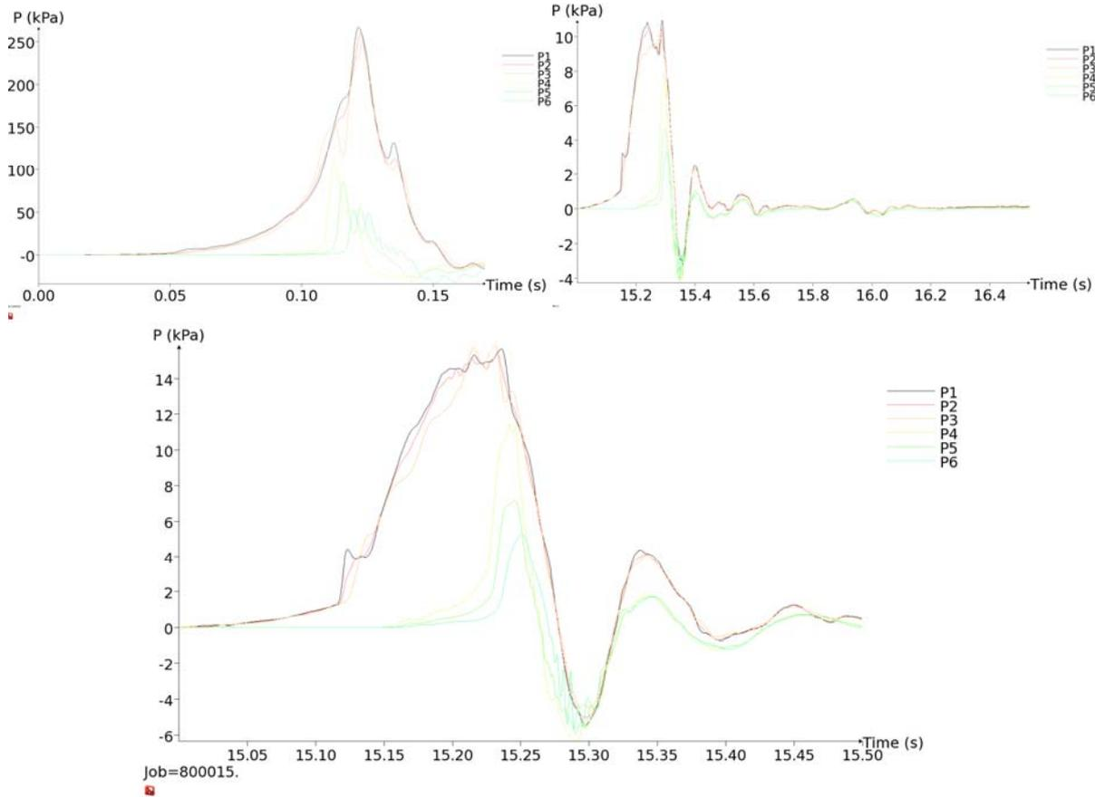
Figure 6 Explosion pressure for realistic worst-case hydrogen (top left), methane (top right) and hythane explosions (bottom). The various curves correspond to six different sensor locations placed inside the garage.
