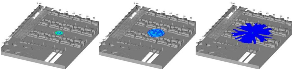
Figure 8 Hydrogen concentrations near the ceiling following a PRD release from a car 0.5s, 1s and 5s after the onset of the release. Vertical structural beams cause the non-circular pattern seen in the middle and in the right picture.
