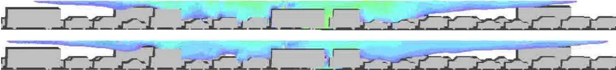
Figure 12 Methane (top) and hythane (bottom) flammable gas clouds 100 s after start of release in the tunnel geometry. The most reactive concentrations around stoichiometry are shown in green.
