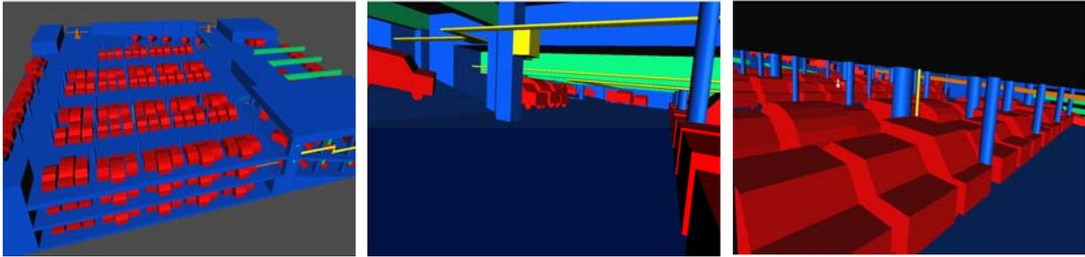
Figure 7 FLACS representation of a three-level underground public parking garage (left picture). The two right pictures show the two different release locations: middle of an open area with flat ceiling (middle) and corner with a lower ceiling and some significant structural beams (right).
