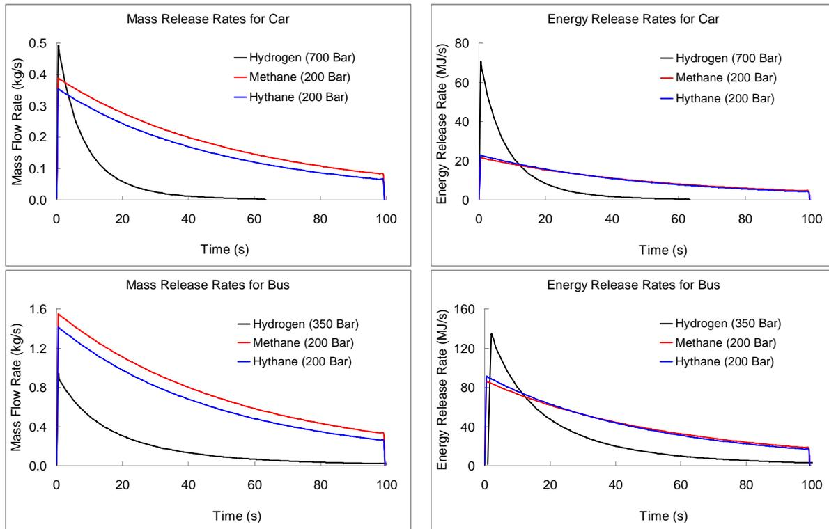
Figure 3 Mass release rates (left) and potential combustion energy release rate (right) for PRD releases from cars (upper plots) and buses (lower plots). It can be seen that even if less mass of hythane is released, the potential combustion energy of the released hythane is marginally higher initially.
