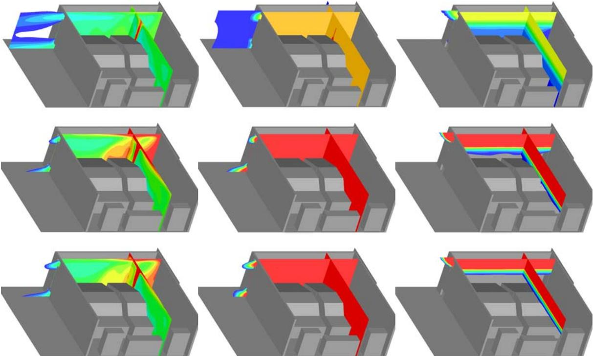
Figure 4 Simulated hydrogen gas clouds 4 s, 20 s and 200 s after start of release (top), methane gas cloud 14 s, 26 s and 500 s after start of release (middle), and hythane gas cloud 14 s, 30 s and 500 s after start of release (bottom). Red colour indicates concentrations at or above the upper flammability limit UFL, whereas green colour is around stoichiometry (most explosive concentration).
