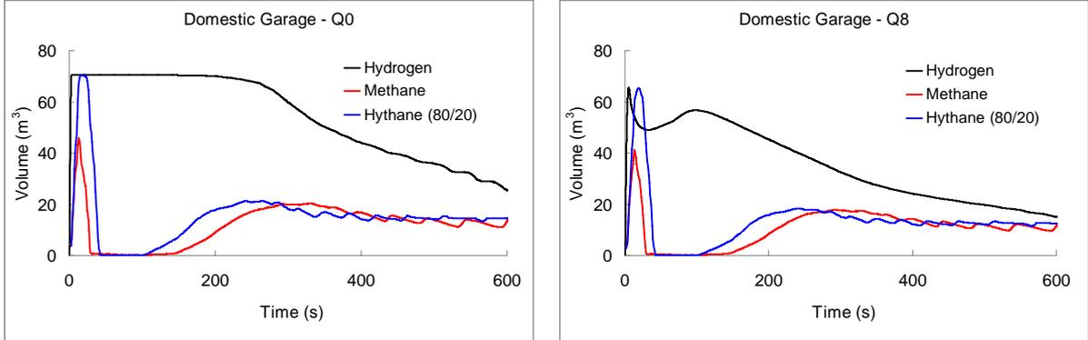
Figure 5 Flammable gas cloud volume (left) and expansion based equivalent stoichiometric cloud (right) for hydrogen, methane and hythane.
