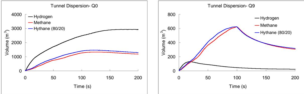
Figure 13 Flammable gas cloud volume (left) and Q9 equivalent stoichiometric gas cloud (right) for hydrogen, methane and hythane mixtures.
