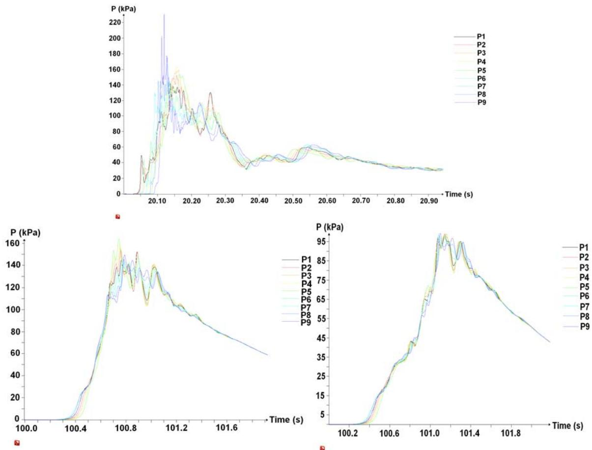
Figure 14 Worst-case explosion pressures with ignition at 20s for hydrogen (top) and at 100 s for methane (bottom left) and hythane (bottom right).
