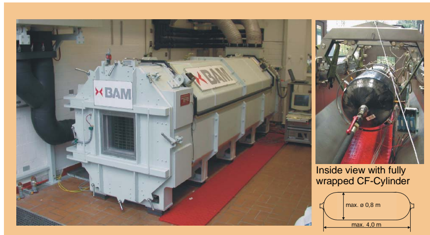
Figure 1. Hydraulic test facility for cycling fatigue and burst tests under extreme temperatures.
